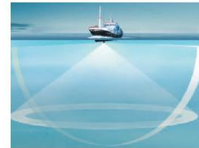
Horizontal and vertical beams The combination of vertical and horizontal presentations show you the schools of fish both from above and from the side at the same time. It is not necessary to go over the target to see the vertical distribution on the echo sounder.
