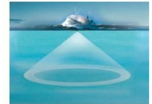
Beam stabilization When the beam stabilizer is activated, both the horizontal and vertical beams are electronically stabilized for roll and pitch. The full circle beam stays on the target independent of the vessel movement, even in rough seas.
